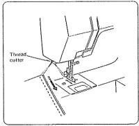
You don't need a pair of scissors to cut the thread after you finish sewing. Just use the handy thread cutter.
